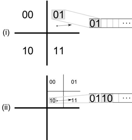
**Fig. 7.** Recursive sort key generation of a single ray for similarity ordering
